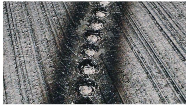
Microscopic 3D image show single engraved dots.
